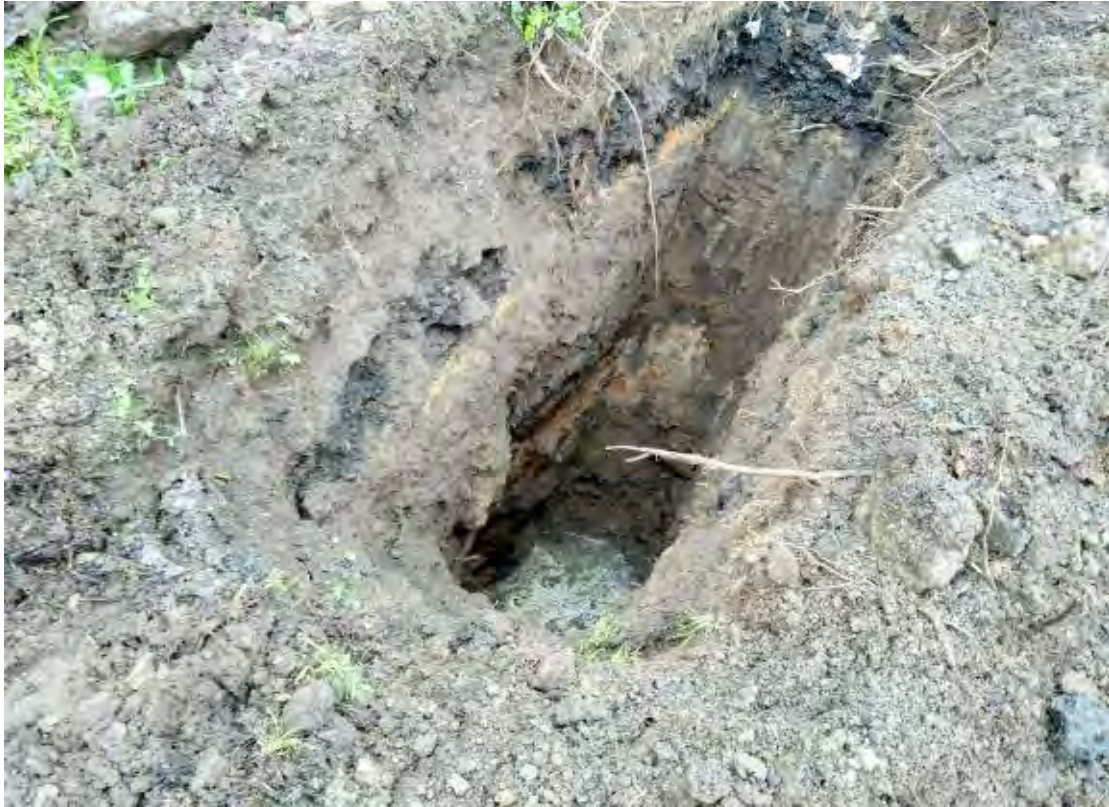
Photo 5: TP124 looking east showing soil profile with groundwater seepage at base of excavation
