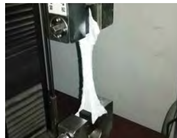
AS 3706.2B GRAB TENSILE STRENGTH
