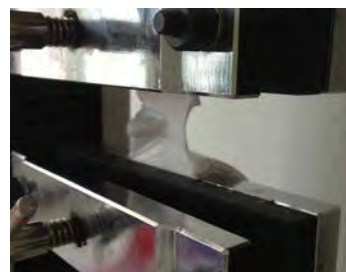
AS 3706.3 TRAPEZOIDAL TEAR STRENGTH
