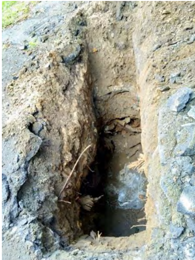
Photo 4: P128 looking east showing soil profile and groundwater at base of test pit
